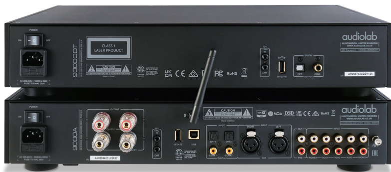
ABOVE: CD transport [top] has opt/coax digital outs and a USB-A port for 44.1/48kHz media on an external drive. Amp [below] has MM, three line ins, a power amp in and pre out on RCAs plus 2x coax/opt digital inputs, a USB-B (768kHz/DSD512) input and main outputs on 4mm speaker binding posts
